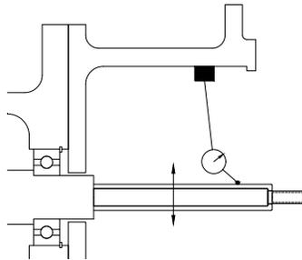
Figure 3: Bearing Fit
